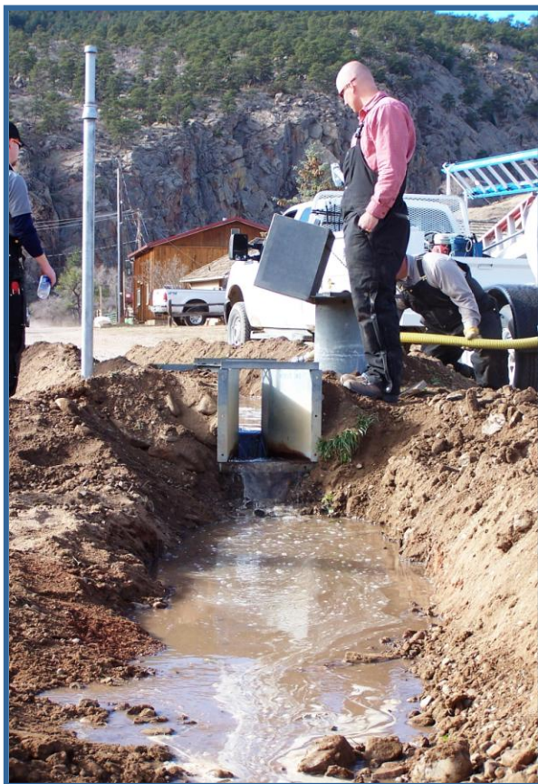
Dave Anderson with Northern Water, oversees a test flow event to get the flume prepared for the Spring stormwater runoff season
